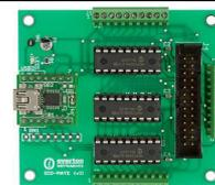
Controlling logic circuits is a common requirement. The two modules above are easy to program, both at the 'bit' and 'byte' levels. The DIO-MATE supports standard TTL logic, while the OPTO-MATE uses photo-couplers to isolate inputs and outputs.
